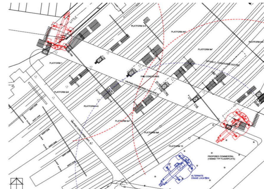
Figure 4 – Possible 450T crane positions showing main boom reach (Note that a local crane contractor was consulted and advised that a 4m heavy duty fly can be added to the main boom if required to increase reach capacity without significantly compromising lifting capacity)
