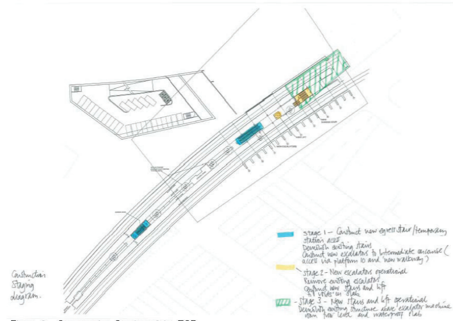
Figure 3 - Construction Staging of the ESR
